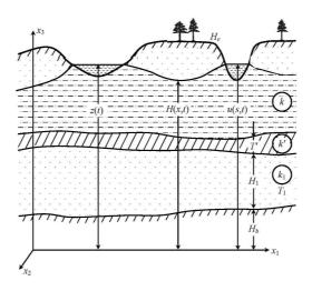
Figure 1: Vertical cross-section of the flow domain. z(t) and u(s,t) are the levels of the water in reservoirs and in the channel. H(x,t) and  $H_1(x,t)$  are, respectively, the groundwater free surface in the upper layer and the piezometric head in the lower layer. k,  $k_1$  and k' are the hydraulic conductivity (percolation) coefficients for the corresponding layers.
