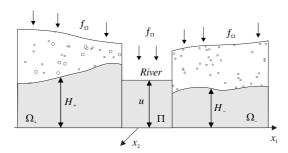
Figure 4: Vertical cross-section in a simplified model.  $H_{\pm}$  are levels of the underground waters on the opposite sides of the river. u is the water level in the river.
