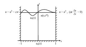
Figure 5: Model of diffusion waves (MDW). Stabilization of the initial level of the water  $u_0(s)$  to a stationary horizontal state  $u^0=cst$ .
