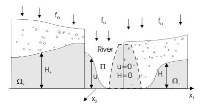
Figure 8: Finite speed of wetting (Coupled Model).  $H_{\pm}$  are levels of the underground waters on the opposite sides of the river. u is the water level in the river.
