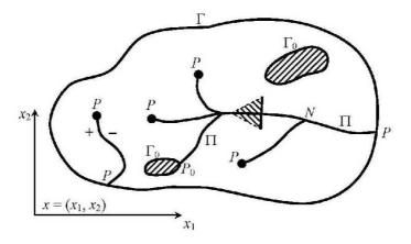
Figure 2: Planar view of the flow domain.  $\Gamma$  is the exterior boundary.  $\Pi$  describes channels or rivers.  $\Gamma_0$  are boundaries of reservoirs.
