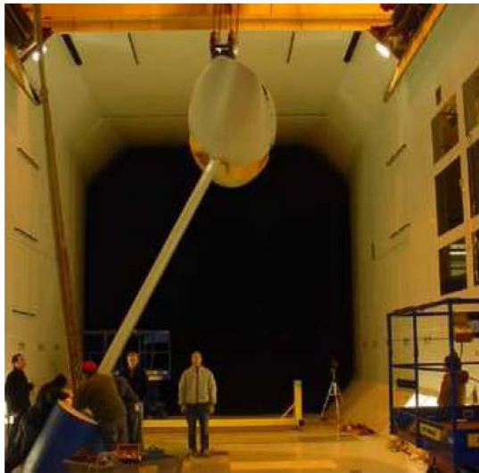
Figure 8: Setup of the 1.5:1 scale model in the wind tunnel.
